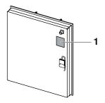
A second identification plate is supplied and should be affixed in the fitted unit underneath the hob.
